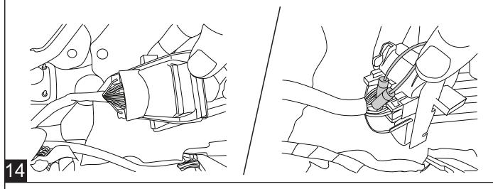
Connect only the purple trigger wire to the OBD II module (#18). Tape off the remaining purple/black stripe wire as it won't be used on this application. Once the trigger wire has been connected to the OBDII module (#18), remove the OBDII port from the vehicle by depressing the two plastic tabs on the sides and push the port back out of the bracket. Now connect the OBDII module to the OBDII port.
