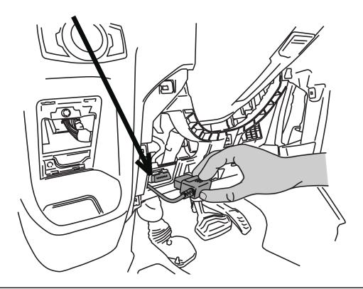
**OBD II install:** Use Supplied Posi-Lock<sup>™</sup> (13) connectors to attach the Plug and Play Module to the Harness. Attach matching colors on the harness to the wires on the module. Plug in module to OBD II port on the vehicle. Secure harness with supplied tie wraps. *Note: If the OBD II pass thru harness (76404-01A) was purchased see install sheet supplied in packaging. The pass through harness allows for an open port for other accessories. See below for a brief description.*
