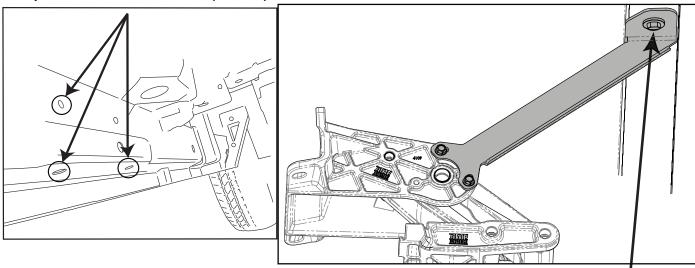
To attach the **Rear Bracket (#21)** to the rear linkage, start by using the Thread Cutting bolt (#23), to cut threads in the blank insert in the frame rail. Use a 9/16" socket and rachet, go slow and stay straight. Then install the bracket on the non-motor side of linkage loosely with two bolts(#22), install the upper Bolt (#23) and Washer (#24), loosely and tighten the bottom two bolts fully. Now, tighten the top.
